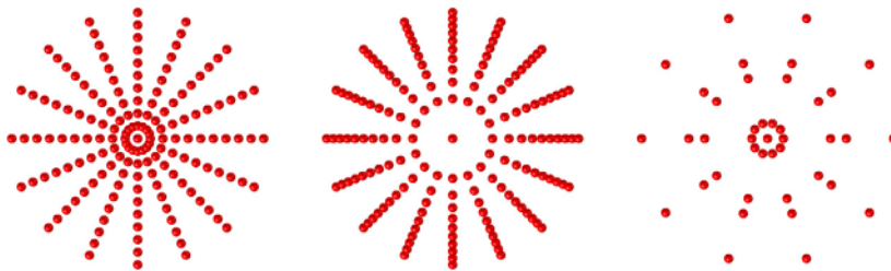
Figure 3-3: Comparison of the cylindrical release in which particles are positioned at uniform radius intervals (left), with uniform number density (center), or at user-defined radii (right).
